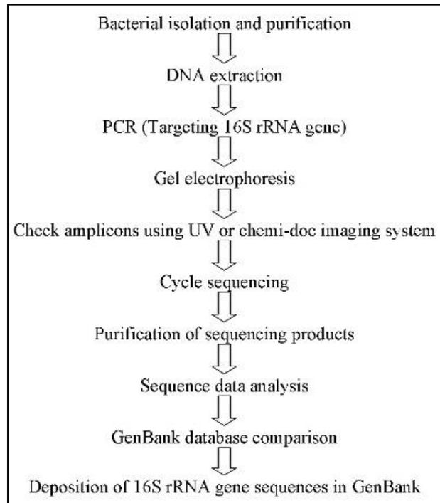
**Figure 1:** Schematic diagram for PCR and 16S rRNA GS-Based identification
